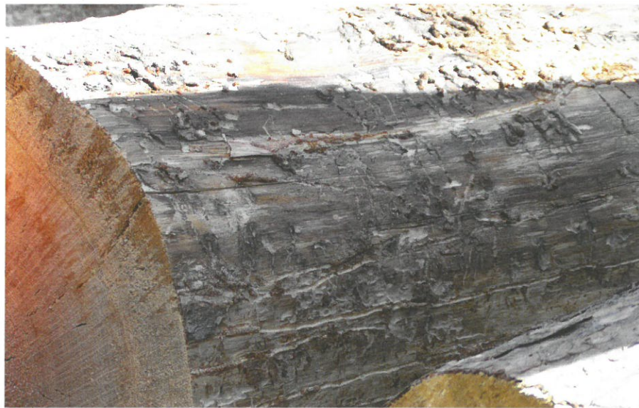
Above: BC Interior pine sawlog showing beetle infestation
